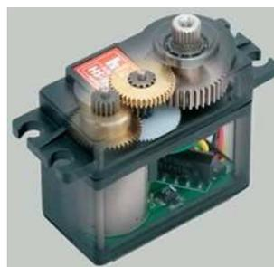
Figura A.14: Servo Motor
